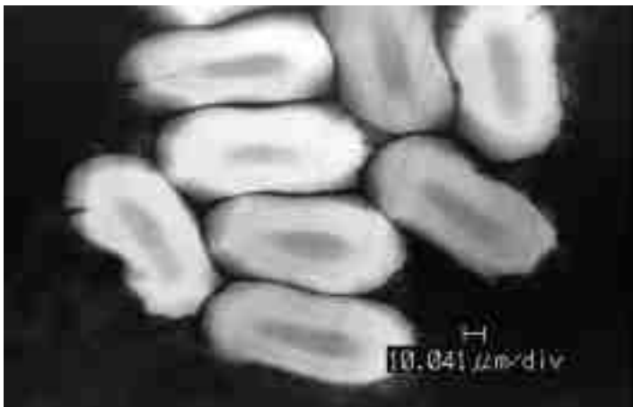
10.11 Dumbbell shape skin/core structure of PVA fiber.
