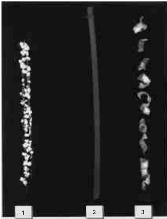
12.18 Extrusion of UHMW PE (1) below the melting point, (2) between 145 and 155°C and (3) above 155°C.
