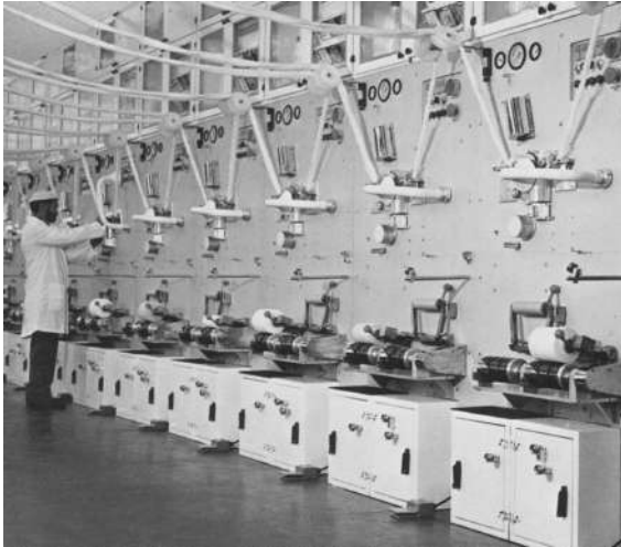
8.8 Bobtex Mark 3 ICS Machine. From publicity material 'Spin at 1000 m/min' supplied to the author by Bobtex International, Leicester, UK.
