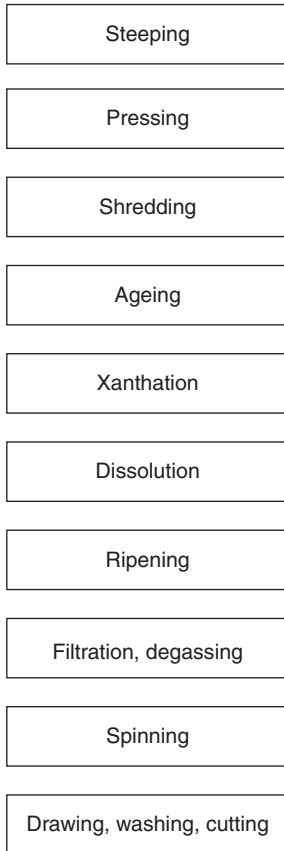
9.3 Viscose fiber production steps.
