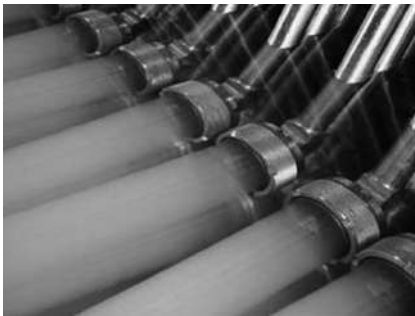
9.2 Extrusion of acrylic fibers from the spinneret. (Source: Courtesy of Akxa, a member of AKKOK Group of Companies, Turkey.)
