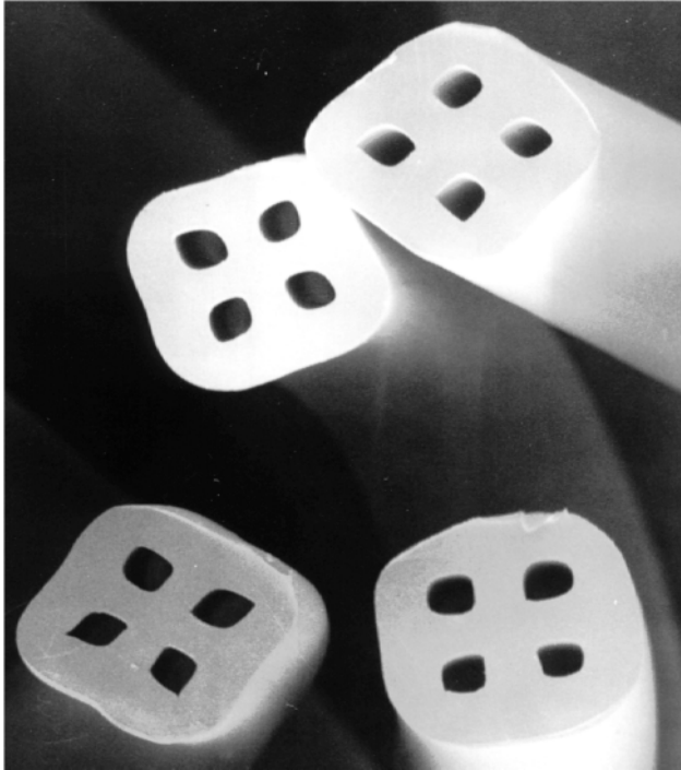
2.7 DuPont Antron ® carpet fibres in transverse cross-section (by courtesy of DuPont Commercial Flooring).
