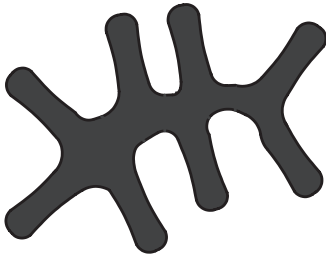
7.4 '4DG' fiber cross-section with deep grooves.
