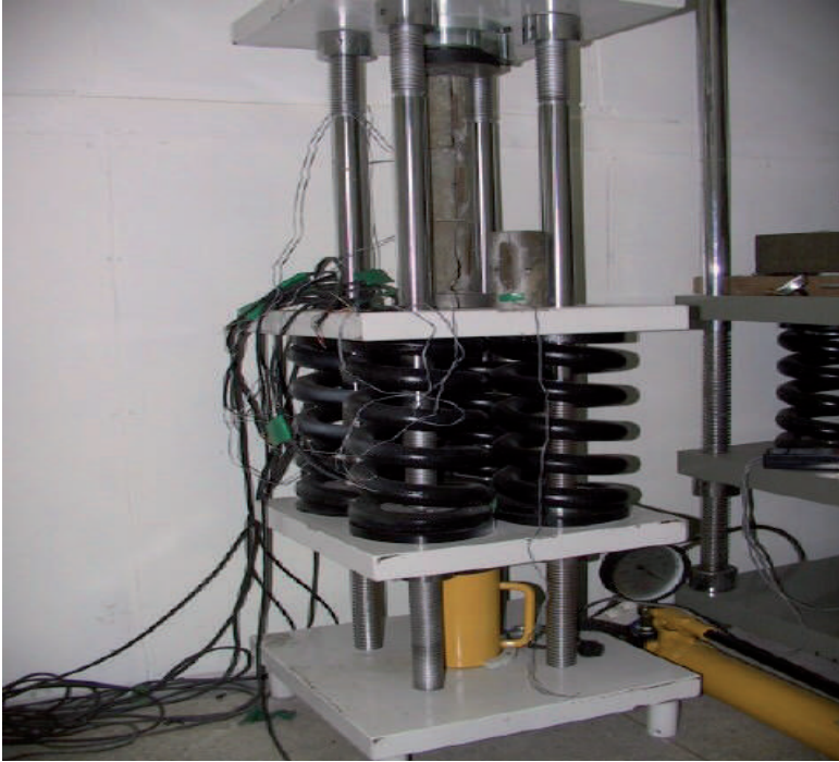
Figure 5. Compressive creep test
