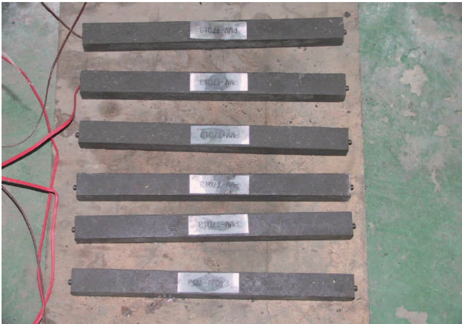
Figure 4. Strain gage setup for length change
