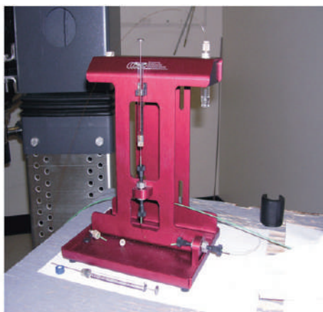
Figure 1. Capillary probe set-up and the Protasis capillary probe injection module.
