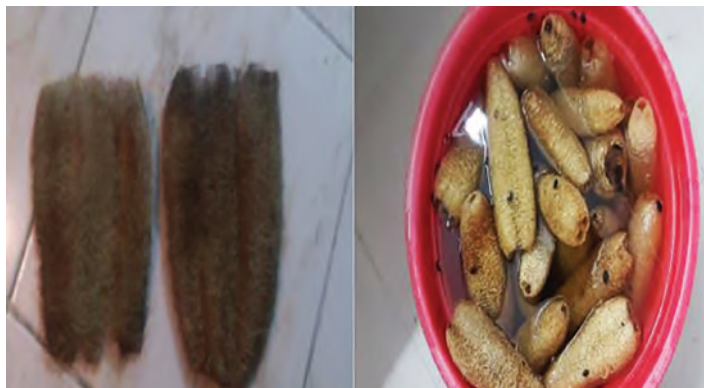
FIGURE 16.5 Pretreatment of luffa fibre with 5% of NaOH.
