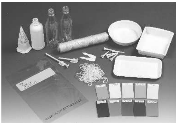
Figure 17.2 Applications of DuPont™ BIOMAX® hydrobiodegradable polyester – film, rigid containers, fibers, injection molded parts and paper coatings. Photograph reproduced by permission of DuPont 1
