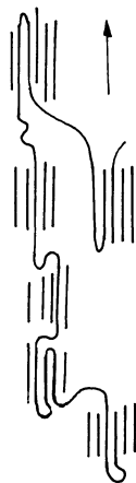
Fig. 2.2 A single molecule may form part of several ordered regions in a fibre.
