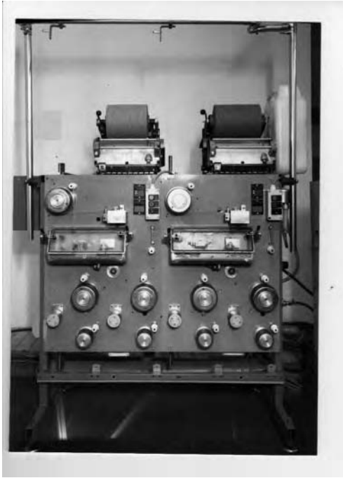
7.2 SSM Eltex Stahl RMT-D air-jet texturing machine. Courtesy of SSM.
