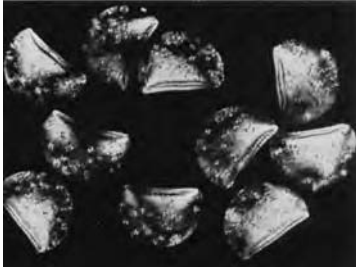
10.1 Filaments from edge-crimped yarn viewed through crossed polars. From Weller (1960).
