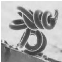
3.1 Monvelle , which was a nylon/elastomer bicomponent fibre, after rupture.
