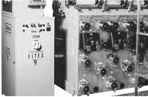
7.3 SSM Stahl DP2-T air-jet texturing machine. Courtesy of SSM.
