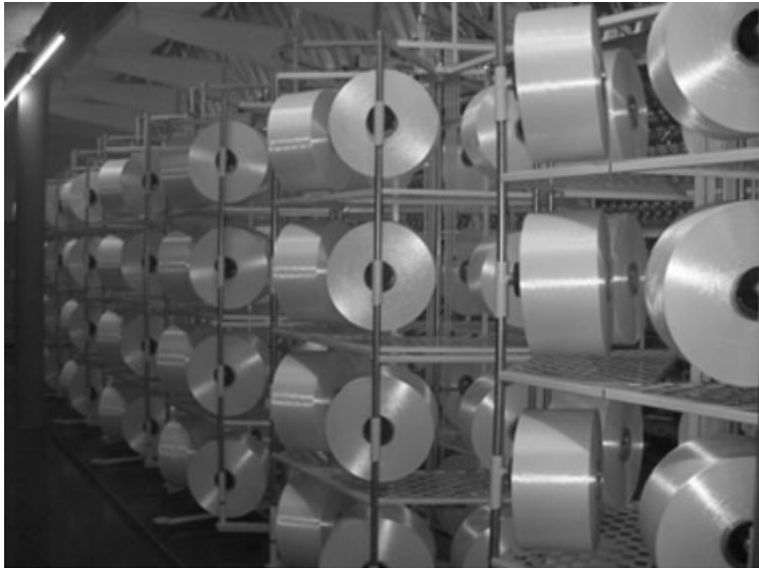
5.16 Four-high rotary creel (Barmag) with protector layer plates.
