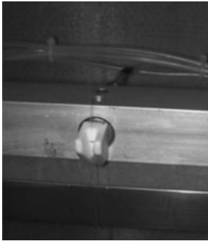
1.8 Ceramic applicator for metered spin finish.
